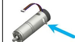
FIG. 1 Motor Retention Screw
